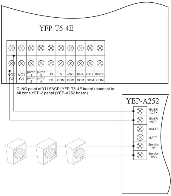
YEP-A252 board: EMER ACT connect to FACP, BATT for standby battery, SPK for speaker.
